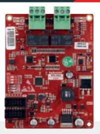
TFC-1201 Loop board communicates with addressable devices over loop line using FlashLink protocol. It has a control capacity of 240 end units.
