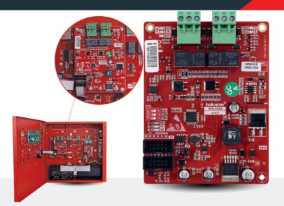
TFC-1201 Loop board communicates with addressable devices over loop line using FlashLink protocol. It has a control capacity of 240 end units.
