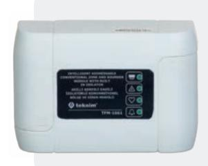
TFM-1661 Conventional Zone and Siren Module is designed to be used with TFP-12xx series addressable fire alarm panels and allows the use of conventional devices in the addressable system, which can transmit alarm and fault information via the loop in a zonal sense and gives a siren output. The device is supports built-in isolator to protect the loop line against short circuit.
