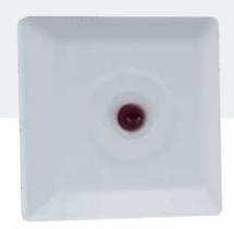
In cases where alarm LEDs are not visible due to installation of detectors on high ceilings, false ceilings, raised floor, restricted access rooms etc., this device is used as an additional indicator light. The big red LED in 10mm diameter can be seen even from high ceiling.
