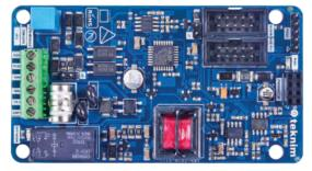
TXM-5270 PSTN module is a communication module designed for the new generation alarm systems of Teknim and designed to send information to the end user or the monitoring center where it is connected with the land line.
