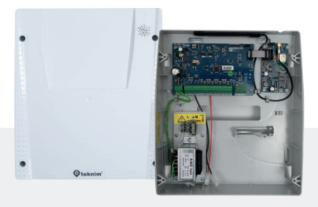
Pars series control panels have advanced protection circuits on the hardware against environmental factors that may prevent the system from working by generating high voltage and current. In this way, the system has been provided to work in a stable manner without deterioration for years.
