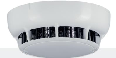
TFD-3230 Conventional Optical Smoke Detector designed to provide maximum level of protection for small and medium sized places with its advanced optical sensing technology. Detector has a series of algorithms developed to minimize faulty detections and to provide pollution warning. Smoke chamber can be easily removed for cleaning in case of possible pollutions in excessively dusty environments.
