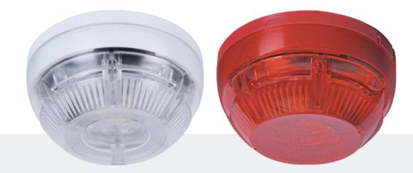
Teknim TFS-1182 is an internal usage fire alarm sounder with flasher and can connect directly to loop line. It can be powered by loop line and has built-in isolator to protect the loop against shortcuts. TFS-1182 supports 42 different tone and 3 different flasher mode options.
