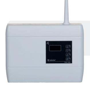
Teknim TWM-1885 Addressable Coordinator is an interface that enables wireless devices such as detectors, MCPs, I/O Modules and sounders to be operated with Teknim addressable fire alarm panels. Teknim wireless fire alarm systems provide a flexible solution by completely wireless or hybrid structure as well as allowing existing wired structures to be expanded wirelessly especially where wiring infrastructure is not possible.
