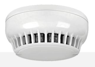
TFD-4230 Conventional Optical Smoke Detector uses advanced Light Scatter technology to detect smoke entering in its chamber. Detector provides maximum level of protection with its advanced optical sensing technology. It has a series of software algorithms to minimize faulty detections and to provide pollution warning. Smoke chamber can be easily removed for cleaning in case of possible pollutions in excessively dusty environments.
