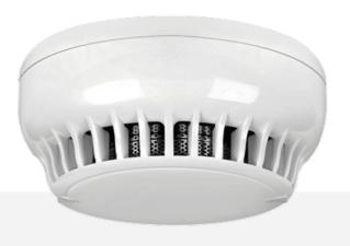
TFD-4240 Conventional Fixed heat detector uses two NTC for precise measurement of the environment to detect fire. Detector classified as A2S and will report an alarm at 55°C.
