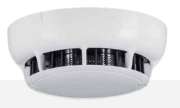
TFD-3245 Conventional rate of rise heat detector designed to detect rapid temperature rise by using 2 NTCs to make an accurate measurement in the environment.
