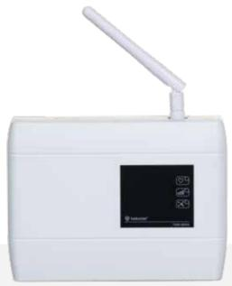
GSM/GPRS dialer is used to deliver alarm information from fire alarm panels to the users over GSM by voice call and SMS and can connect directly with the Alarm Receiving Centers to deliver alarm information via GPRS. It can also be used to remote start/stop of a product connected over PGM output via SMS. It can be used with all brand of fire alarm panels.
