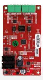
TFC-1209 Network Module establishes a strong ring or bus network by inter-connecting 16 panels via TdNET protocol. It also supports built-in isolator which helps to protect the network line in case if there will be a short cut at the cable between control panels.
