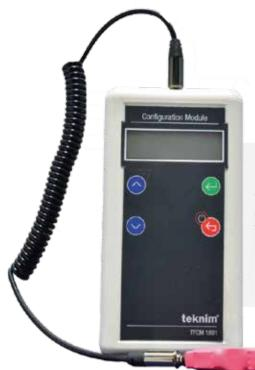
TFCM-1801 device programming module is developed to define address for addressable devices such as detectors, mcp, input-output modules or to read defined address and firmware version of the devices. It is supplied from 9V (6LR61) battery.
