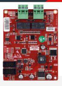
TFC-1201 Loop board communicates with addressable devices over loop line using FlashLink protocol. It has a control capacity of 240 end units.
