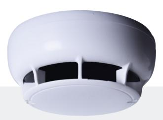
TFD-3245 detector uses two NTC and digital processing algorithm to measure the environmental temperature. Detector works as A2R class which sense a quick rise in temperature and also a fixed tresholds temperature of 55°C.
