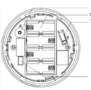
Link/Test Button CR123A Battery Tamper Switch
