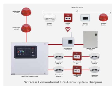
TWM-1885 Wireless Addressable Coordinator can only be used with Teknim brand addressable fire panels, while the TWM-3885 Wireless Conventional Coordinator can be used with all brands and models of conventional fire panels. In this way, you can design a project completely wireless as in addressable or conventional, you can expand a previously installed system with wireless products, or you can create a hybrid structure by designing the project both wired and wireless from the beginning.
