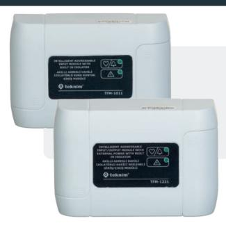
**TFM-1011** supports single monitored input and can be used with TFP-12xx series addressable fire alarm panels. The device is also supporting built-in isolator to protect the loop line against short circuit.
