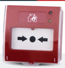
TFB-1166 is an addressable manual call point with built-in isolator, designed and produced comply with EN54-11 and EN54-17. It is equipped with dual LEDs to indicate local alarms (Red Colored LED) and short-circuit alert (Yellow Colored LED). TFB-1166 MCP can be used with TFP-12XX Addressable control panels through Flash Link protocol.
